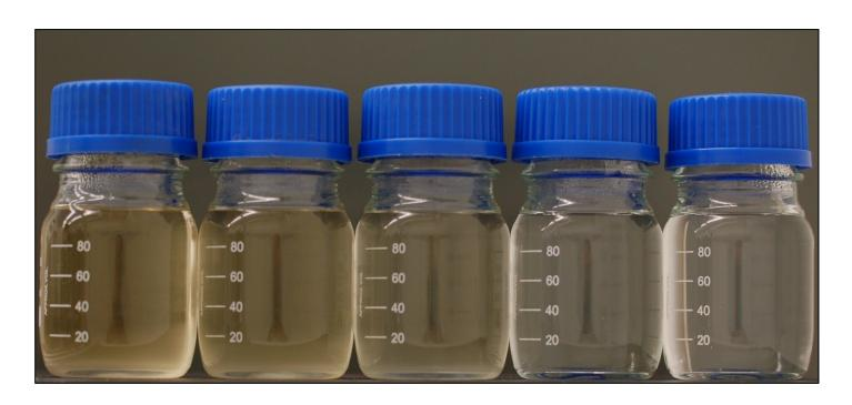
Scale precipitate at left (90:10, 75:25, 50:50 water 1:water 2)
