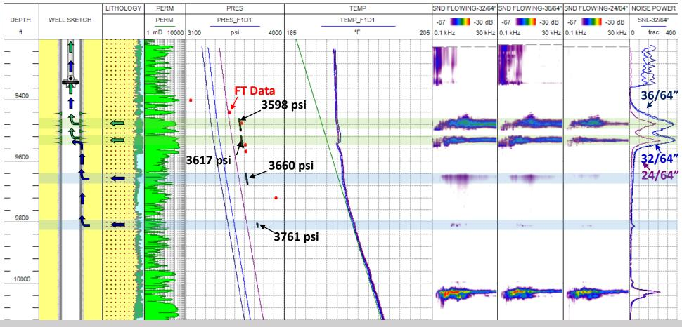
In this case study formation pressure of 3 zones is determined by Noise Logging, including 2 zones behind the casing (cross flow), this data was then compared with existing Openhole data with great accuracy.
