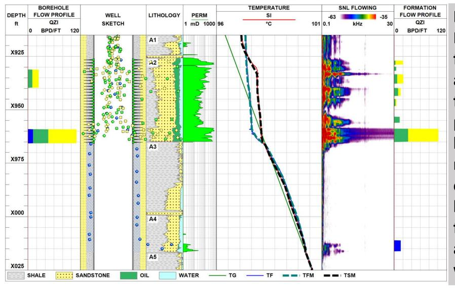
In this case study, **PLT Spinner shows in** flow of both water and hydrocarbon from the perforations at A2, but the Noise response reveals a channelling flow behind the casing from A4 which is the actual source of water.
